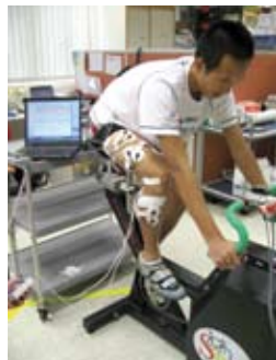
Fig 1: Surface EMG was recorded continuously from 8 muscles of the right leg during the 5-minute cycling exercise
